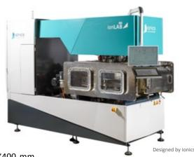
The ionLAB equipment allows ion implantation of flat surfaces of 400X400 mm controlled by an automated XY table. The system is equipped with one or two ionGUN's 2000: an industrial ion source able to use different gases and to reach ion beam currents of several milliampere with accelerating voltages up to 40 kV.
