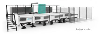
The ionPRO industrial line is dedicated to the treatment of large flat parts with the innovative ion implantation technology. Five ionGUNS 2000 arranged in line ensure the efficiency and homogeneity of the ion implantation treatment. The lock chamber is composed of two loading plates allowing a continuous treatment in the process chamber. The treated surface area reaches 1600x1800 mm with a maximum speed of 150 mm/s.
