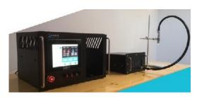
The ionJET is an atmospheric plasma torch based on a new flexible microwave technology. Unlike RF torches, the plasma is generated at the outlet of the torch. The active species directly
